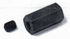
Simply thread tool on 5/16-24 end of stud about  $1/2^{\infty}$  in depth, then piace ailen set screw so it bottoms on top of stud. Use a 5/8 socket on a 3/8 ratchet to drive coarse end (5/16-18) of stud into hole.
